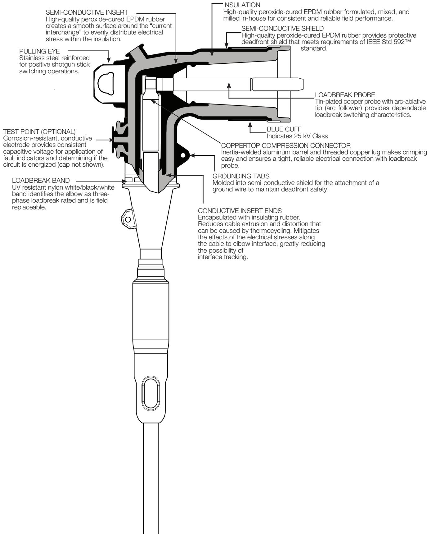
Figure 2. Elbow cutaway illustrates design features.
